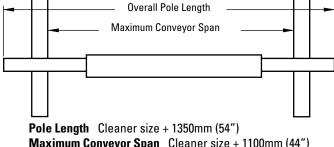
Maximum Conveyor Span Cleaner size + 1100mm (44")
